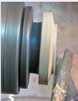
5 Turn away wood with a gouge, beginning to shape the convex face to half the depth of the recess.
