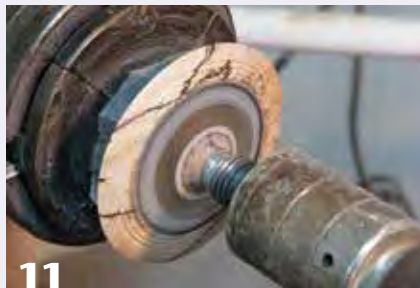
11 Turn away the tenon and bottom layer of wood. With the tailstock in place, a nub will remain that cannot be turned away. Here, I left a large nub, but it can be much smaller if you use a cone on the live center.
