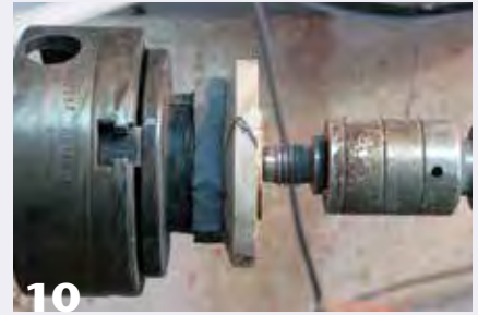
10 An alternative to the vacuum chuck: press the workpiece with the tailstock live center against a soft pad held in a chuck.
