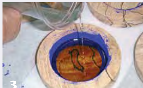
3 Pour epoxy into the recess until it is half-full.
