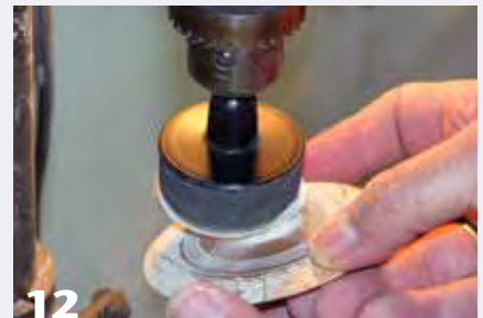
12 Sand away the nub using a sanding attachment chucked in a drill press.
