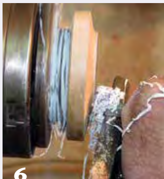
6 Use a negative-rake scraper to turn the epoxy window. Don't worry, it will be well worth the stringy mess.
