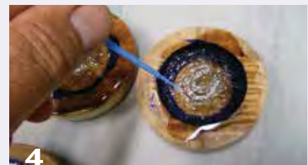
4 Add decorative elements such as mica, then complete the epoxy pour to the top, trapping the sparkly materials inside what will become a translucent window. Reposition errant pieces with a small pick or brush.
