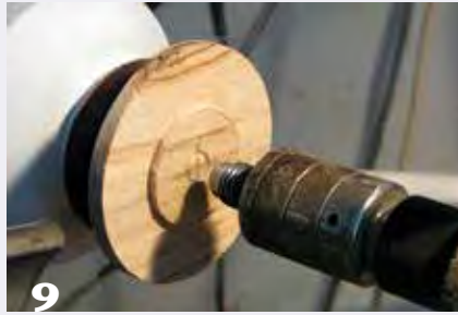
9 Reverse-mount the ornament so you can turn the opposite side. I like to do this with my vacuum chuck, using the live center for alignment.
