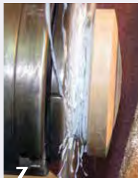
7 The finished convex shape of one side of the ornament.
