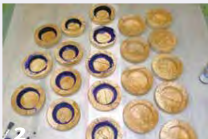
2 Paint the inside walls of the recess. Any paint on the recess bottom will be turned away later.
